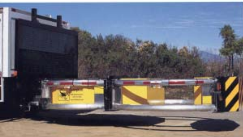
The Scorpion TMA is fully extended, with the chargeable message panel in the travel or storage position.
