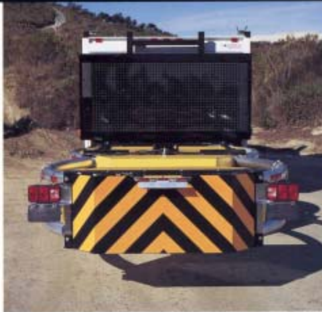
Rear view of the Scorpion TMA fully extended along with the message panel in the down storage position.
