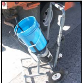
Place the 5 gallon pail on the Roklin Motorized Pail Mixer, ensuring the pail is secure in the correct slots.
