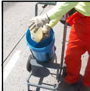
Pour the contents of bottle "A" into the 5 gallon pail making sure it doesn't splash out.
